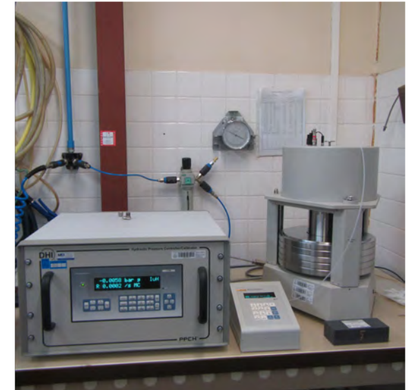
Shom's automated mass handling piston gauges and calibrator CPC 8000
