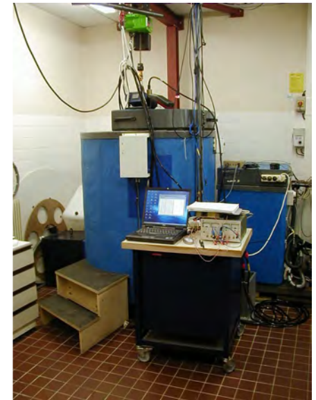
Shom's calibration bath and one salinometer
