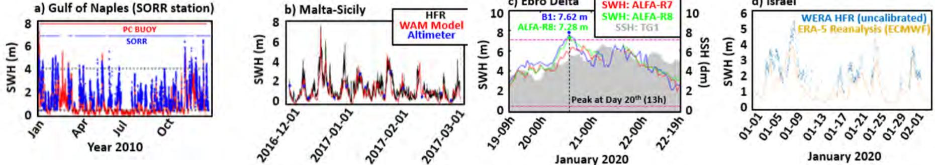
Time series of the validation of HFR derived Significant Wave Height (SWH) versus: a) PC buoy (in the GoN); b) WAM model and altimeter (in Malta-Sicily Channel); c) buoy (Ebro Delta); d) ERA-5 reanalysis (Israel)
