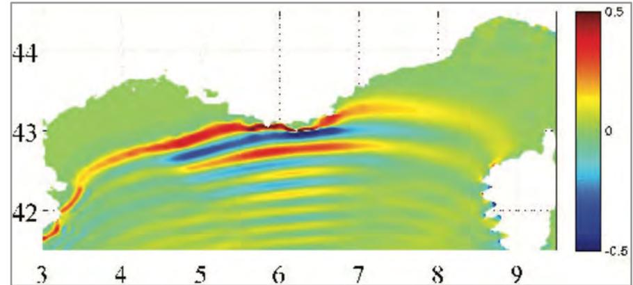
Simulated surface elevation (in meter) after 1h10 propagation for a tsunami generated by a M7.8 seismic source in the North of Algerian margin (courtesy of Stephan Grilli, Univ. of Rhode Island, USA).
