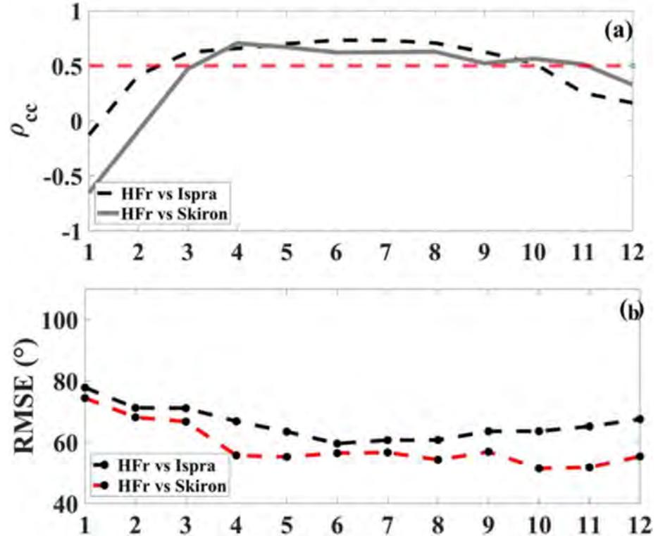
Variation of the (a) circular correlation coefficient and of the (b) RMSE on range cells between HF radar wind direction versus the weather station (located at Ispra) and the model SKIRON/Eta for February 2009 in the Gulf of Naples. Saviano et al., 2021
